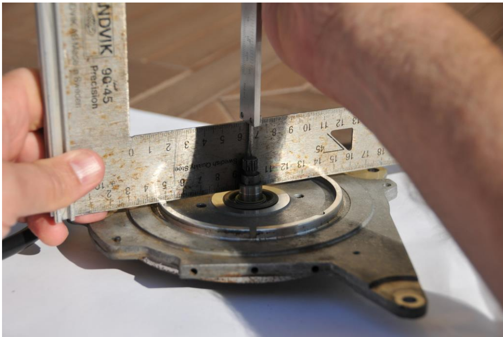
Original Optispark axel. Length from reference surface 20,2mm
