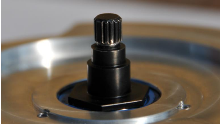
Close-up pictures of MSD spline turned 360 degrees
