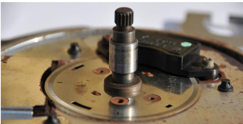
Original spline axel fits perfect into the female spline without any force.
