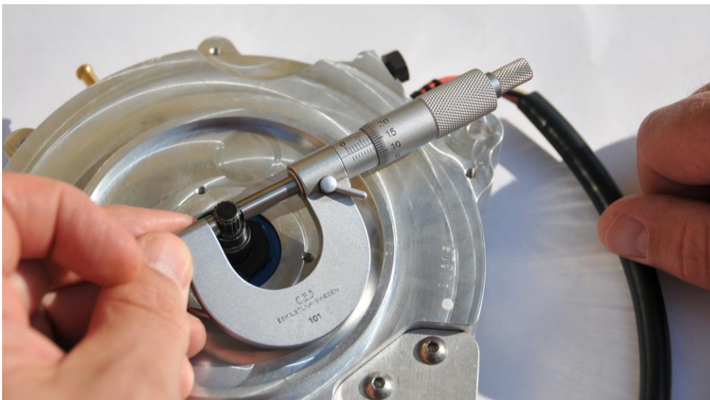
MSD Optispark axel. Outer diameter 8,14mm to 8,22mm depending on measuring on top or between spline.
