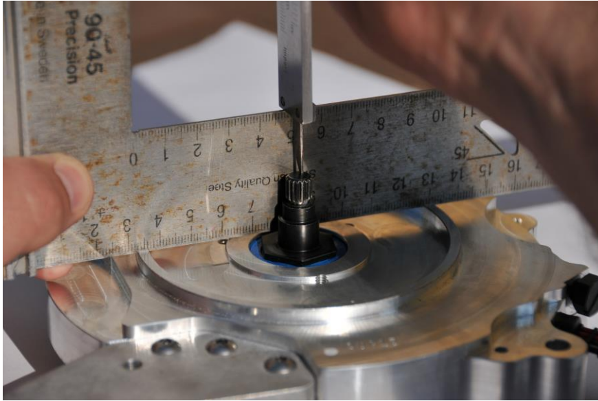
MSD Optispark axel. Length from reference surface 20,8mm
