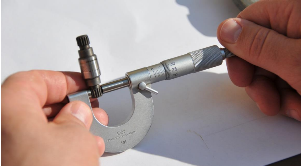
Original Optispark axel. Outer diameter 8,25mm to 8,40mm depending on measuring on top or between spline.
