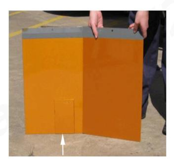
This photograph shows the same paint test panel with a slight crease in the center, creating an angle in the panel similar to the Camaro door to quarter panel relationship. The finish on the right side of the panel has "shifted", creating a different hue of the same color. Note the arrow shows the paint standard on the left side of the paint test panel in the same position as the first photograph.
