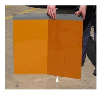
This final photograph shows the same paint test panel described in the second photograph. In this photograph, the arrow points to the same paint "standard" used in the first two photographs but it has been repositioned to the right side of the paint test panel. Note the paint "standard" has shifted along with the finish on the paint test panel.
