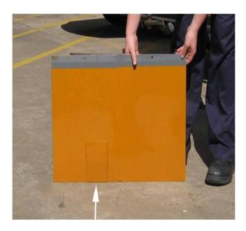
This first photograph shows a paint test panel finished in "Wildfire" metallic. The white arrow points to the paint "standard". This is the paint sample used to ensure color consistency.
